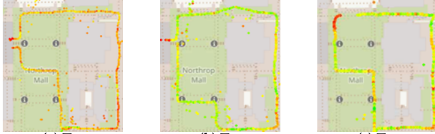
Figure 32: Sample throughput traces collected at a location with bad coverage at different times of the day. The green color indicates good throughput.
