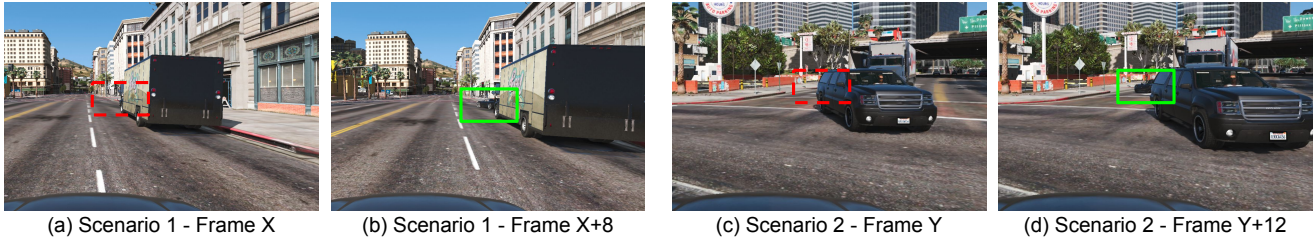
Figure 16: Image data collected by the ego-vehicle in two scenarios where EMP detect road hazards earlier.
