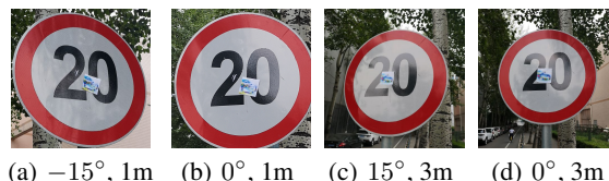
Figure 7: Traffic signs with adversarial patches on them. The photos are taken in the campus of Beihang University with different distances and angles using camera. Traffic signs are respectively classified as “No Entry”, “Slippery Road”, “Speed Limit 60” and “Over-weighted Vehicles Prohibited”.
